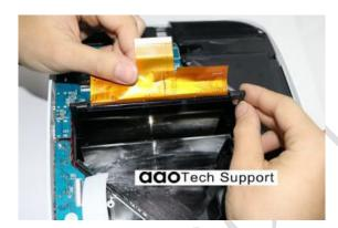
7. Remove the old screen. When removing the screen, please refer to the technique of the picture to avoid fingerprints. Besides, take care if the direction of the screen when removing.
