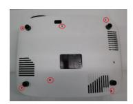
2. Gently pry the cover up by finger or tools, turn it over and remove the button cable.
