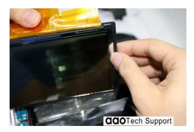
The front of the screen faces the light cup; to align the card slot like picture 3; Avoid fingerprints on the screen.
