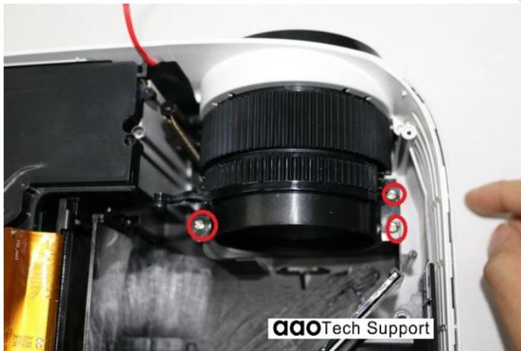
11. Remove the lights path cover, screw back the 4 screws .
