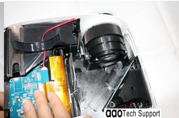
**7. Note: Must turn the lens focus wheel to the left as picture 1; Remove the whole lens like the gesture of picture 2**
