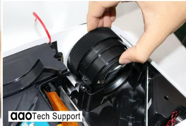
**8. Recover the Lens Put the lens back in place like picture 1, then screw the focus wheel to the right like picture 2;**
