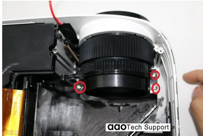
6. Remove the Lens : Don't pick up the keystone correction wheel, just press the keystone correction wheel on the picture. Gently lift it up and remove it.
